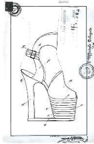
10 Patent 19736, February 12, 1941: sandal with layered platform sole and connection between heel and sole.
